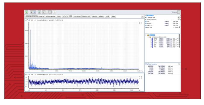
When higher resolution and frequency range are required for FFT with symptoms, EVAM, SPM HD Expert or SPM Spectrum, e.g. when monitoring high-speed gearboxes in turbines, MOD194 extends the maximum of these parameters. The lower frequency limit is then 0, 0.5, 2, 10 or 100 Hz. The upper limit is 40 000 Hz. The number of spectrum lines can be extended to max. 12 800 or 25 600.
