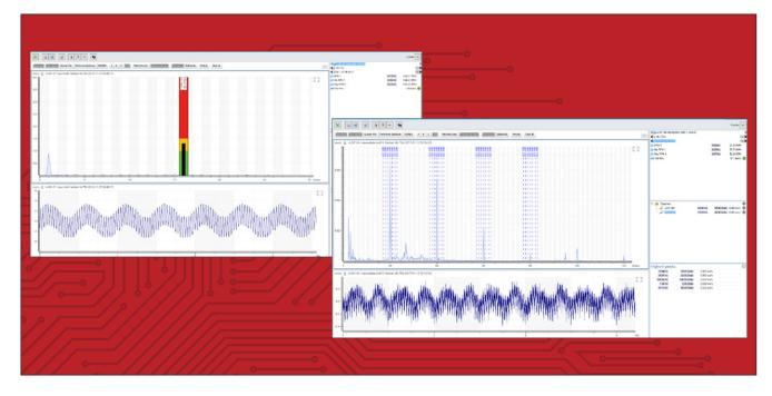
FFT Spectrum with symptoms is a vibration analysis function offered with Leonova and Intellinova. It is a reduced form of EVAM (TD-591), lacking the statistical evaluation by means of criteria.
