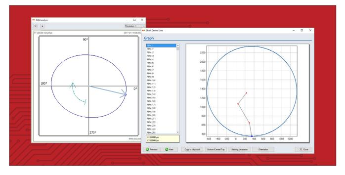
**Orbit Analysis** is a vibration measurement function offered as a module for Condmaster Ruby. The resulting orbit graph shows the movement of the shaft's centerline and is used to detect failures like rubs, unbalance, misalignment or oil whip on machinery with journal bearings.
