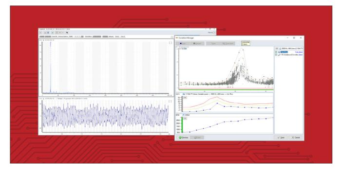
With Leonova and Intellinova, EVAM (Evaluated Vibration Analysis Method) is offered as an analysing function. The method generates three sets of machine condition data:
