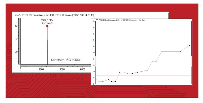
Broadband vibration measurement is the most widely used and cost-efficient method for the diagnosis of general machine condition.
