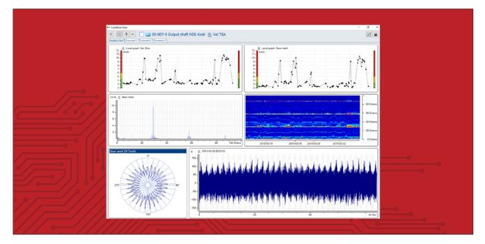
Condition View is a flexible and powerful function that makes it possible to combine multiple graphs in Condmaster into a single window for presentation and further analysis. The function can be used to show current machine condition, recent condition development or maintenance actions, e.g. to clarify or justify planned maintenance activities.
