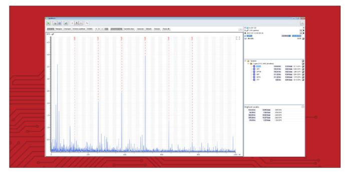
The SPM Spectrum measuring technique is a complement to the SPM dBm/dBc and LR/HR techniques. The purpose of SPM Spectrum is to verify the source of high shock pulse readings. Shocks generated by damaged bearings will typically have an occurrence pattern matching the ball pass frequency over the rotating race. Shocks from e.g. damaged gears have different patterns, while random shocks from disturbance sources normally do not coincide with the pattern of the machine element of interest.
