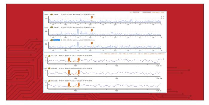
Multi-channel simultaneous vibration monitoring, including both two-channel and three-channel measurements, is a module function in Condmaster Ruby that requires either 'FFT with symptoms' or 'EVAM' to be active.
